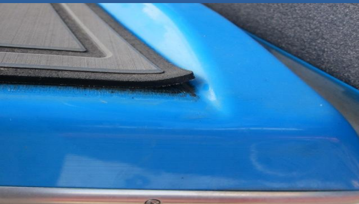
The corners and edges of some swim board mats are pulling up.
