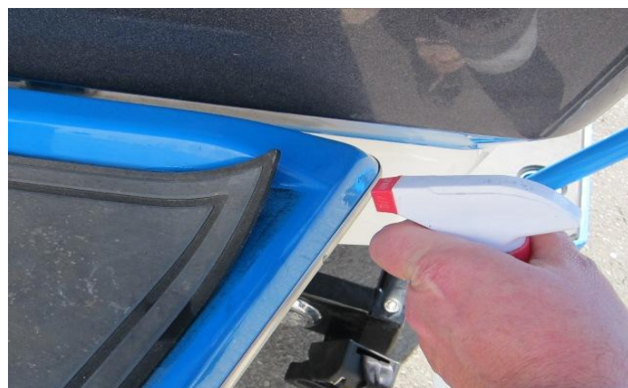
Apply alcohol to the exposed area of the swim board. Wipe off with a clean rag to remove surface debris.
