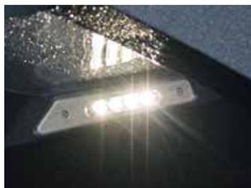
**Courtesy Lights:** The courtesy lights vary from model to model and are found in all areas of the deck from bow to stern, as well as inside storage compartments. (Lights in storage compartments are controlled separately.) Also available as an option are under-seat courtesy lights.
