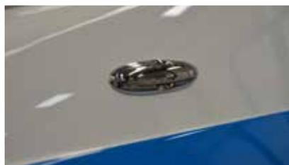
**Cleats:** All boat models offer optional pop-up cleats. Where equipped, the cleats will be located below the windshield on each side of the deck, and also near both rear sides.
