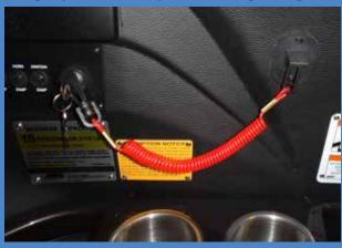
The Emergency Safety Lanyard is designed to turn off the engine whenever the operator moves far enough away from the helm to activate the switch. The purpose is to stop the engine, propeller, and boat in the event the operator leaves the helm location, falls overboard, or is ejected from the boat. If the engine is stopped it will prevent the boat from becoming a runaway, unmanned boat, which may cause injury or death to boat occupants who have fallen
