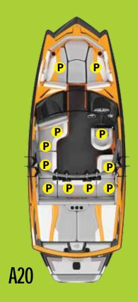
The seating chart is provided to aid in safer boating. What is shown is the maximum capacity in terms of people on board. As more gear is added, the number of people must be reduced to avoid a situation in which the boat could potentially capsize.
