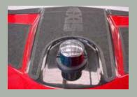
open the pop-up, push down on the chrome exterior and the light will pop open. To close, push down on the light and it will fold into the deck casing.
