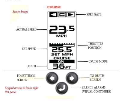
**Cruise Mode:** This information shows the current status of the Cruise Mode. When it is turned on and engaged, the cruise control system will automatically control the speed of the boat after the actual speed has reached the desired set speed. (The cruise ON/OFF is located on the lower right side of the instrument panel.)
