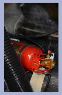
An automatic fire extinguishing system has an LED-lighted indicator located adjacent to the throttle-shifter at the driver helm. As part of the routine safety checks as the boat powers up, the operator should verify that the extinguisher system indicator is active.
