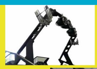
The tower on all Axis models is the Grey Skull. The Grey Skull can be raised to its full height for extraordinary boating enjoyment, or lowered for towing and storage, or for bridge clearance while on the water.
