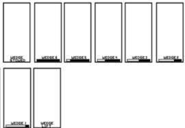
A wedge storing screen appears when the wedge is moving from the maximum wedge position to the stowed position. It will flash at one-second intervals as the action is performed. A buzzer also sounds but can be silenced by pressing Enter.
