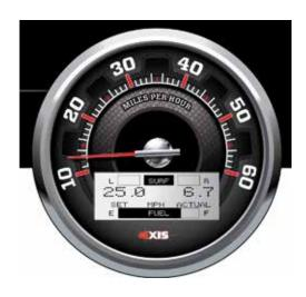
The Axis tachometer has an alpha-numeric display that allows the user to access both boat and engine information. The toggle switch is located on the tachometer. Some information such as the depth and GPS may not be present, depending upon whether a depth module or PGS puck has been installed.
