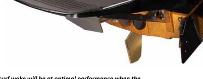
methods for creating a surf wake, with Surf Gates the surf wake will be at optimal performance when the boat is weighted evenly. If too much ballast, gate and passengers are loaded to one side or the other, it could create an unstable situation in which the boat could become swamped. Always use common sense and good judgment in adjusting weight on and in the boat.
