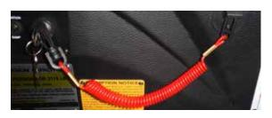
There are practical limitations to what the Emergency Safety Lanyard can do. It can take several seconds for the engine and propeller to stop turning. The boat can continue to coast for several hundred feet depending on the boat speed at the time the switch is activated. While the boat is coasting, it can cause injury to anyone in its path. Accidental loss of power can be hazardous particularly when docking or in heavy seas, strong current, or high winds.
