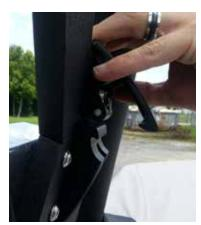
To raise or lower the tower, Axis strongly recommends a second person to help steady the tower into position. The tower's weight could cause loss of control, resulting in damage to the boat or potential injury to person(s).
