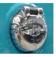
Axis boats are equipped with fuel fill fittings and vents to provide state-of-the-art safety protection in the process of adding fuel to the tank. While most of the fuel system on the boat is inaccessible to owners/operators, the fuel fill was designed to ensure the process of fueling up is as safe as possible and efficient.
