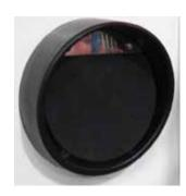
Some flaps and components of the exhaust system are composed of highgrade rubber and synthetics. These may deteriorate over time. Check to ensure that the flap fits securely over the exhaust port and that it opens with ease, which is what must occur when the boat engine is running.
