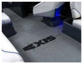
The carpets and mats available through Axis are constructed of durable, marine-grade material. Occasionally washing with a mild detergent (such as Dawn dishwashing soap) and warm water is required. Commercial carpet cleaners (such as Woolite Spray Carpet Cleaner) are also acceptable.
