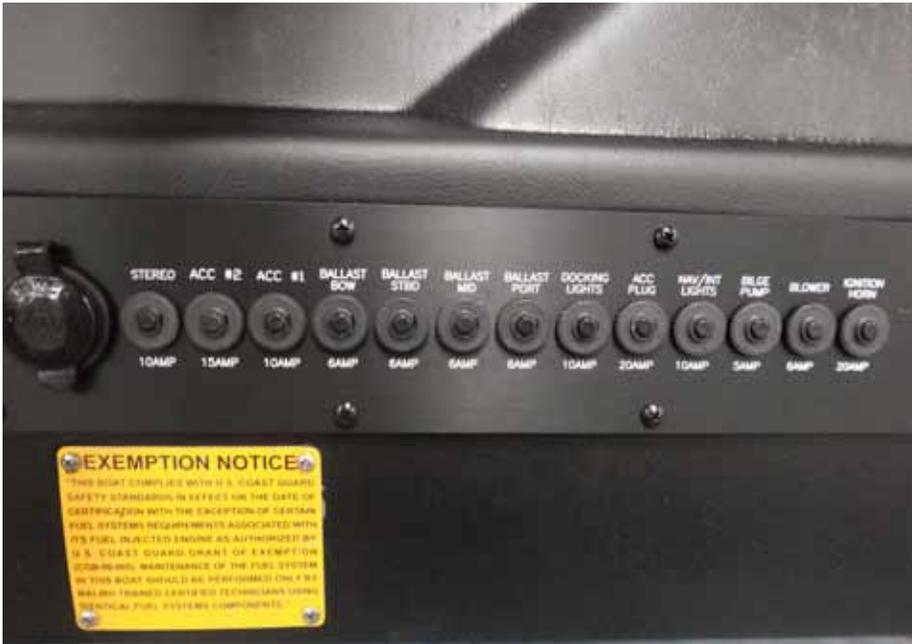
Figure 2-2. Circuit Breaker Panels
