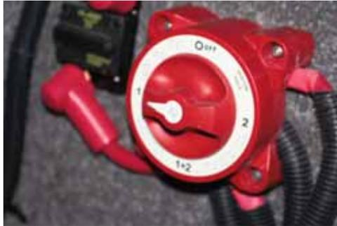
**Figure 4-8. Battery Switch**
