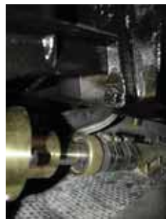
Figure 4-1. Dripless Shaft Seal
