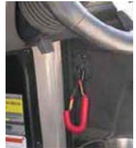
Figure 2-6. Emergency Engine Stop Switch
