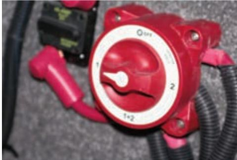
**Figure 4-8. Battery Switch**
