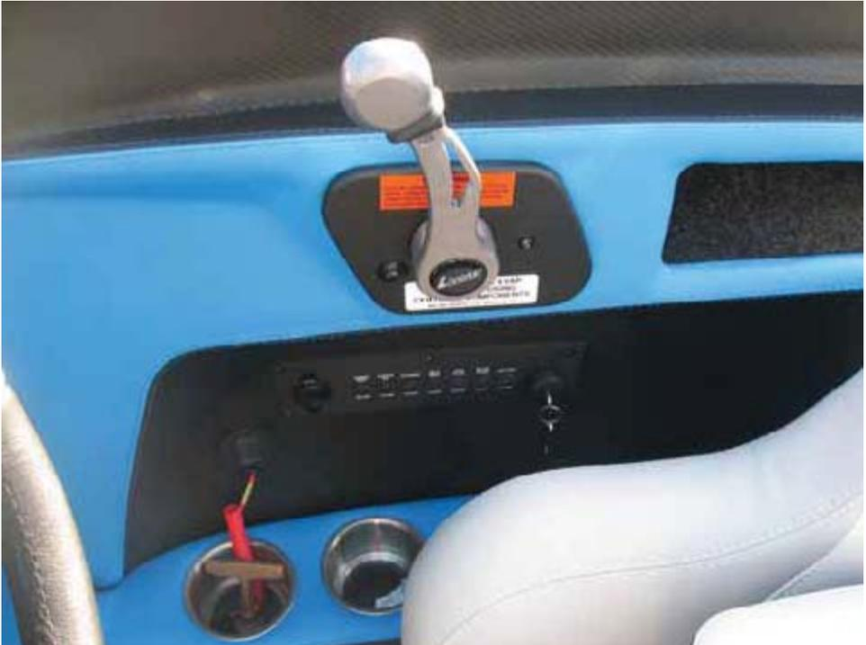
Figure 2-2. Circuit Breaker Panels
