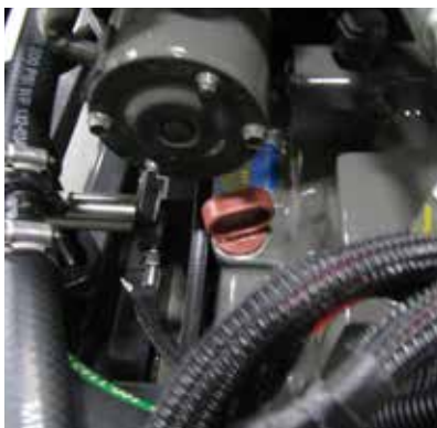
Transmission dipstick (red); V-Drive dipstick (yellow).
