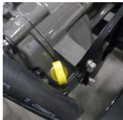
Transmission dipstick (red); V-Drive dipstick (yellow).
